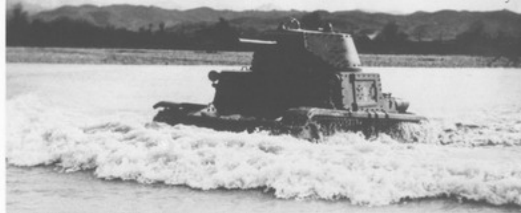
An M 13-40 assigned to the IV (4th) Tank Battalion crosses a shallow river in Italy during a training exercise. This tank could ford streams up to 39.4 inches (100.1 cm) in depth; however, it was not equipped for wading in deep water. The IV Battalion trained extensively in Italy before it was deployed to Albania in late 1940. (LUCE, via Cappellano)
