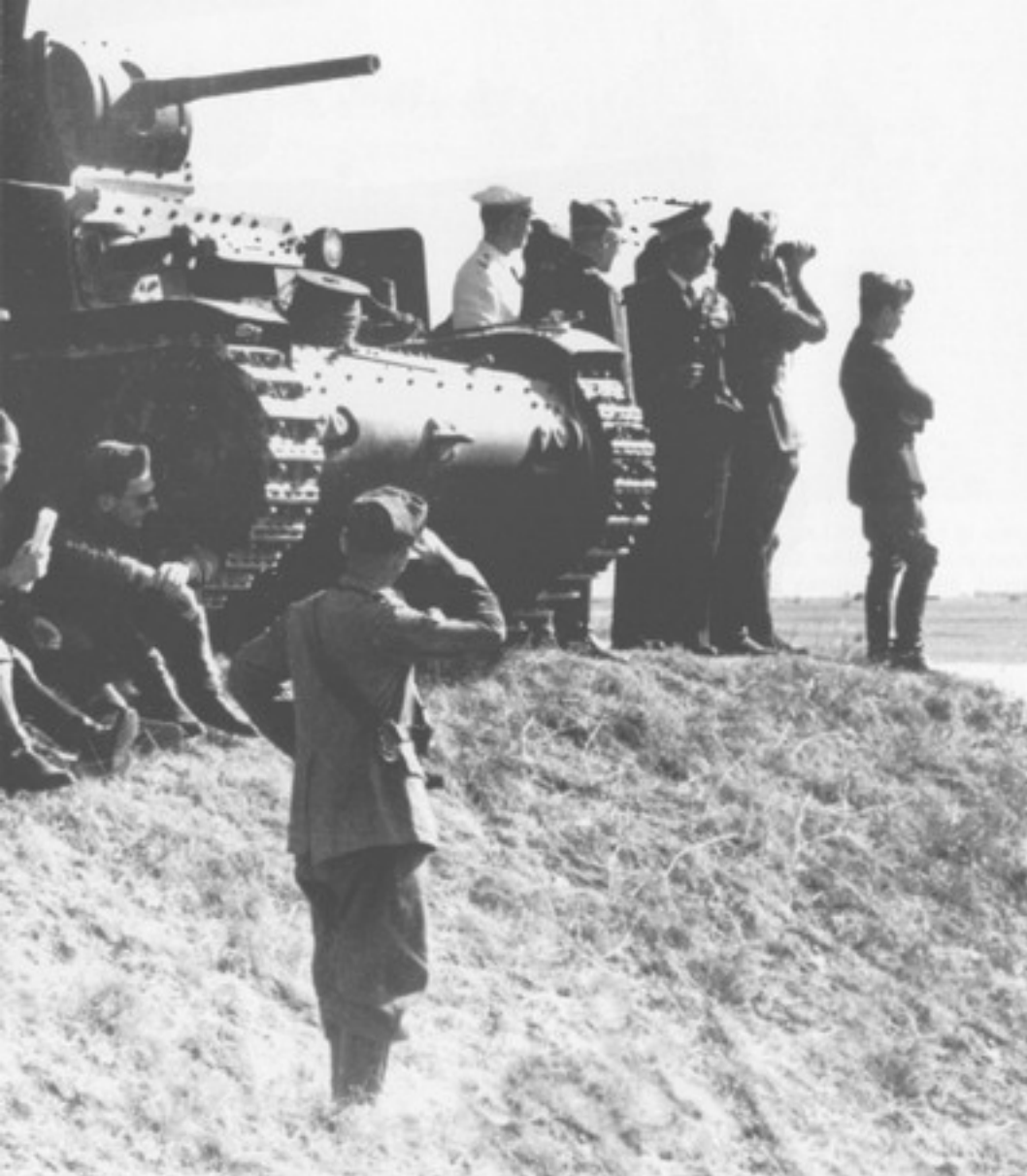
This M 13-40 was used by Italian officers as a communication post during an exercise. A reel of telephone wire was placed on the front hull before the twin machine gun mount and open driver's hatch. The Regio Esercito (Royal Italian Army) were issued gray-green service uniforms in Europe; however, both gray-green and tropical khaki uniforms were worn by Italian personnel stationed in North Africa. (Cappellano)
