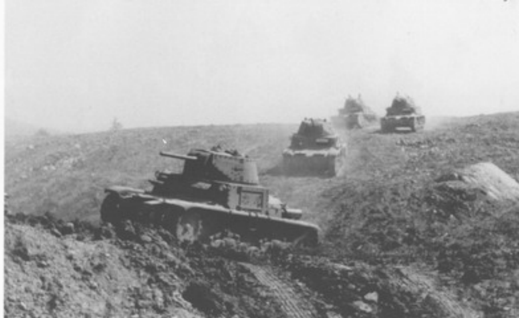
Production M 14-41s perform testing at the Ansaldo Proving Ground during 1942. These tests confirmed the new tank's performance and handling over the type of terrain likely to be encountered on the battlefields of North Africa and Europe. The M 14-41 – like the earlier M 13-40 – could cross trenches 6.9 feet (2.1 m) in depth. (Rosini)
