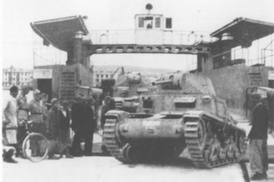
The last M 14-41s deployed to North Africa were landed at Bizerte, Tunisia in late 1942. They were immediately sent to face the British and American forces closing in on the Germans and Italians. The M 14-41 retained the 47mm turret-mounted gun and the two hull-mounted 8mm machine guns fitted to the earlier M 13-40 tank.
