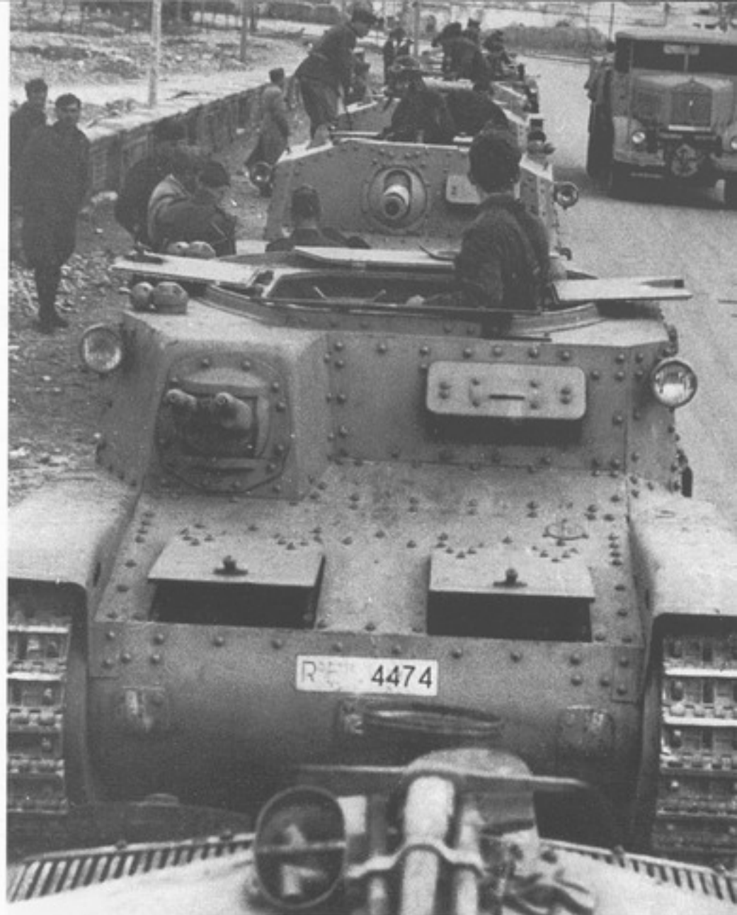
A Carro Comando based on the M 13-40 chassis (R 0 E 70 4474) leads a battery of Semovente da 75/18s in Tripoli, Libya in January of 1942. These vehicles were assigned to the first Semovente unit deployed to North Africa. The early command vehicles used the twin 8mm hull machine gun mount used on the M 13-40 and M 14-41 tanks. A crewman stands up in the Carro Comando 's fighting compartment, with all four of its hatches opened. The pioneer tools placed on the near vehicle's engine deck were a pickaxe (top), a shovel (lower right), and a crowbar (lower left).
