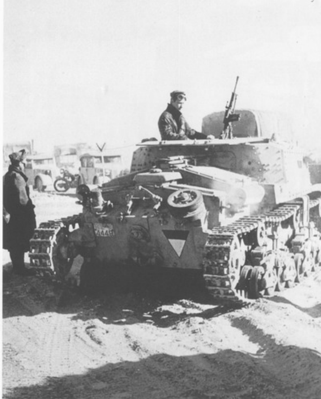
A loader stands in the fighting compartment of a Semovente da 75/18 (R 0 E 10 4449) in North Africa. A 6.5mm Breda Model 30 machine gun for anti-aircraft use was fitted to the fighting compartment roof. This weapon was replaced by the 8mm Breda Model 38 machine gun on later production Semoventi . The yellow and black assault gun tactical marking was repeated on the rear hull plate. A track connecting tool for installing track links was mounted on the aft hull, between the jack and the spare bogie wheel.
