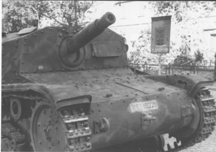
This Semovente da 75/18 (RE 16225) was parked on an Italian street sometime in 1943. The 'pepperbox' muzzle brake fitted to the 75mm gun diverted some gas expelled with the projectile when the gun was fired. This gas was turned to develop a forward thrust in order to counteract some of the gun's recoil, which otherwise moves the weapon backward. The vehicle was delivered to the 31st Tank Regiment at Siena, Italy on 31 May 1943. (Bundesarchiv)
