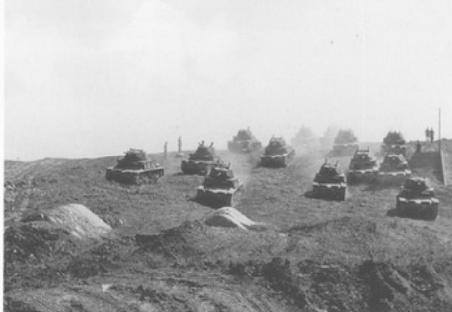
A company of M 14-41s charge downhill during testing at Ansaldo's Proving Ground near Genoa, Italy during 1942. Most of these tanks have their two-piece turret hatches opened. Each M tank battalion consisted of three companies of 15 tanks each, with seven additional tanks assigned to battalion headquarters. (Rosini)
