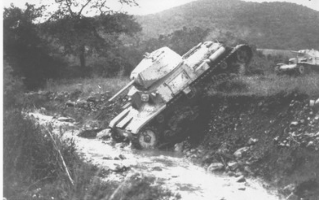
A battalion of new M 13-40s train in Italy for fighting in North Africa during the spring of 1941. Beginning with the 752nd vehicle produced, the M 13-40 was fitted with shorter fenders and different footsteps on both the port and starboard sides. (AUSSME)
