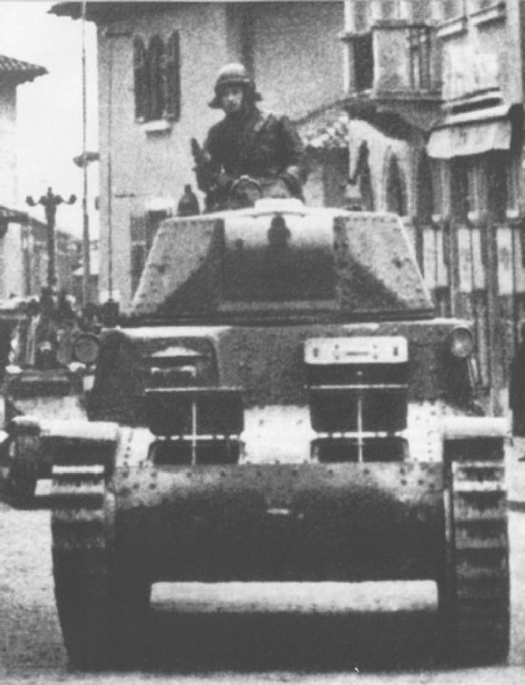
One of the Littorio Armored Division's few M 13-40s crosses the Yugoslav border at Sussa on 12 April 1941. The commander sits on the turret roof with little threat of enemy gunfire present. Both brake inspection hatches were propped open on the tank's bow. This Division was based in northeast Italy and advanced along Yugoslavia's Adriatic coast to reach Ragusa (now Dubrovnik, Croatia) on 17 April. (Pignato)
