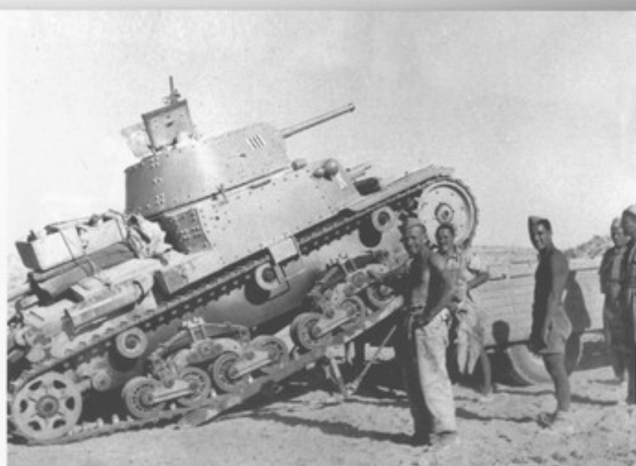
Italian armored personnel unload an M 13-40 from its transport trailer in North Africa. The tank used a ramp mounted to the trailer's aft end for loading and unloading. The white turret rectangle indicated the tank's assignment to the regimental headquarters company, while its three black stripes signified the Company's 3rd Platoon. (LUCE, via Cappellano)
