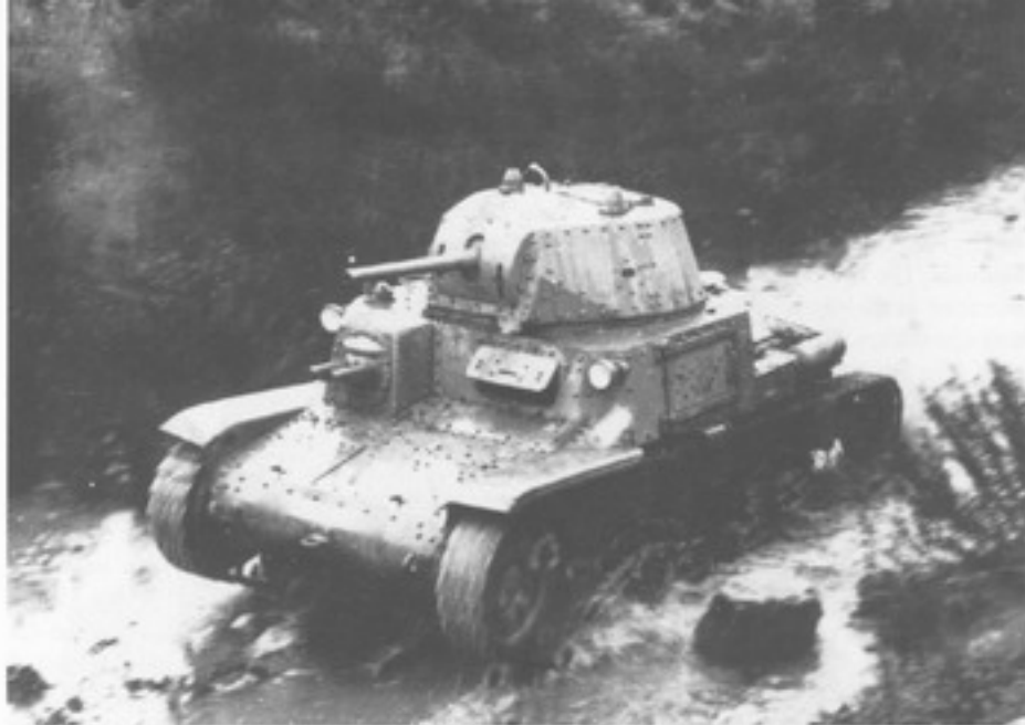
An M 13-40 on training exercises rides through a narrow Italian stream during the spring of 1941. The driver has opened his hatch for an improved view of the territory ahead of his tank. M 13-40s produced from early 1941 were painted overall Yellow Sand (FS20260) instead of the previously used Gray-Green (FS34159). (AUSSME)
