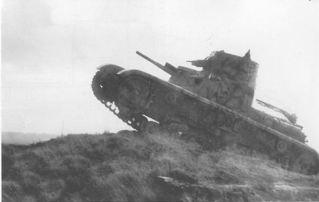
The Fiat-Ansaldo 8 T prototype performs mobility tests on difficult terrain in 1937. This tank (redesignated M 11-39 in 1939) had a ground clearance of 1.3 feet (.41 m). The two turret-mounted 8mm Breda Model 38 machine guns were pointed downward while the M 11-39 climbed up this slight hill. (AUSSME)
