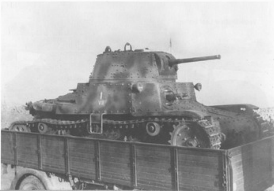
A tank officer stands beside an M 13-40 (R o E o 3052) during his training period. Armored personnel wore red and sky blue collar patches on their gray-green uniforms. The Royal Italian Army's vehicle registration number was only displayed on a stamped plate on the tank's left rear before mid-1941, when this number was also painted on the front hull. The registration was in red lettering and black numbers on a white background. (Palma)
