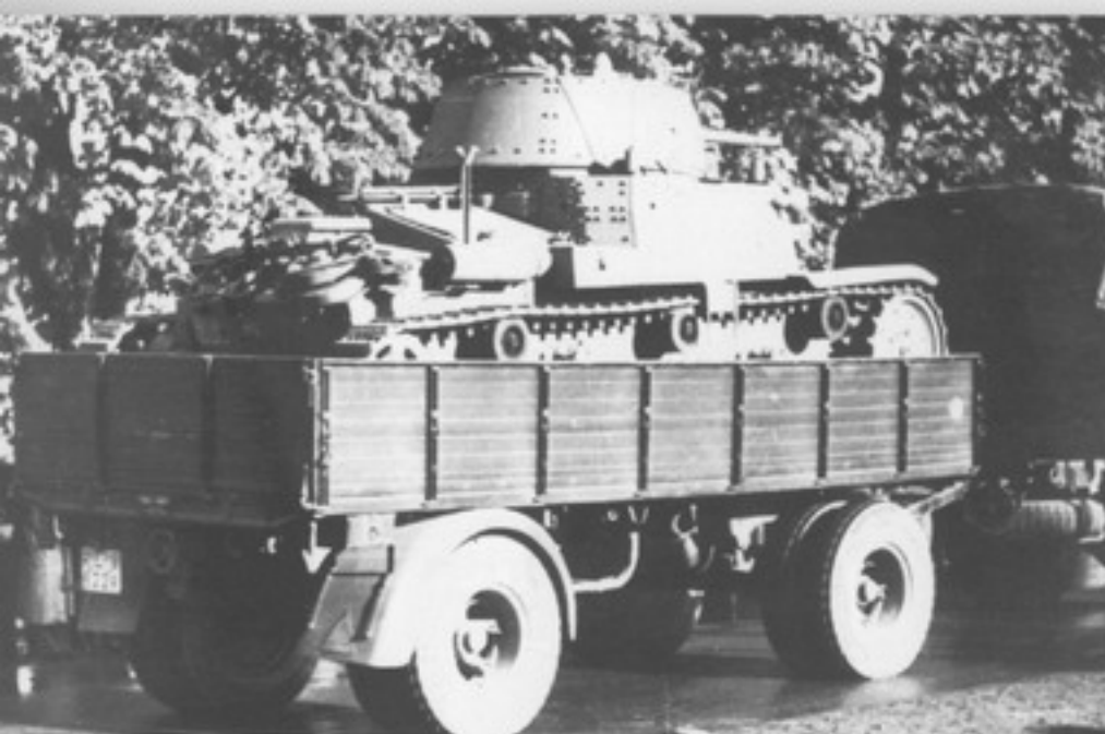
An M 13-40 Centro Radio (Radio Center) command tank is parked on a transport trailer connected to a 3/40 truck during a wartime parade. The Centro Radio variant was equipped with RF 1 CA and RF 2 CA radios for use by battalion commanders. The two radio antennas were mounted to starboard of the turret. (AUSSME)
