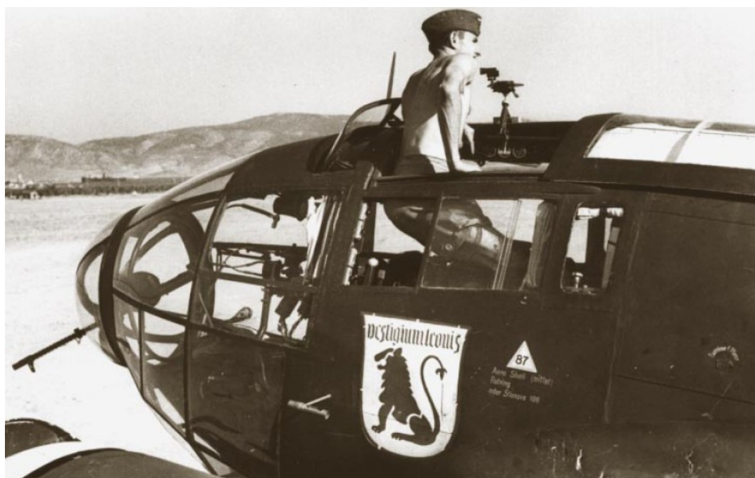
Fig15. The Plath Sun Compass in use calibrating compasses in a German Heinkel 111 bomber plane. North Africa, 1940's. After Konrad Knirim.
