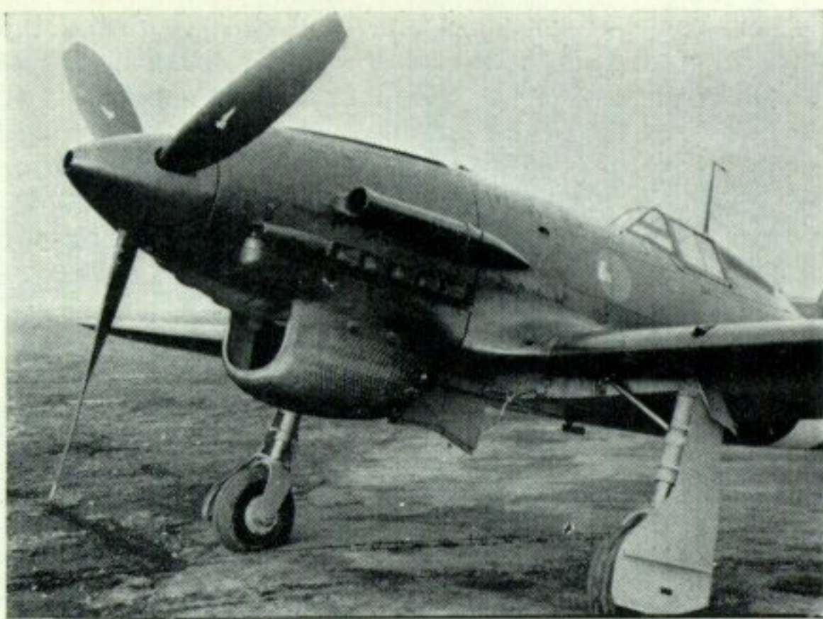
Close-up MM7768 showing the experimental chin radiator.
