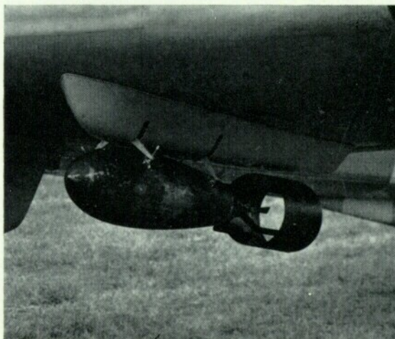
Close-up of tail-armed 250-lb. bomb on Hurricane II.
