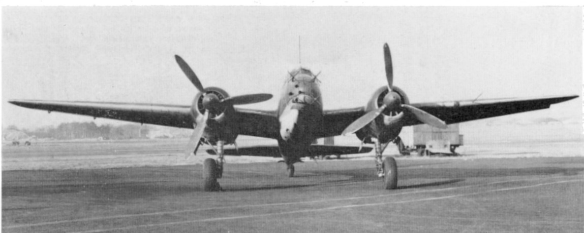
Head-on view of the Ju 88R-1; apart from the substitution of air-cooled BMW engines for the liquid-cooled Jumo 211's, this variant was identical to the Ju 88C-6b. (Photo: Crown copyright)
