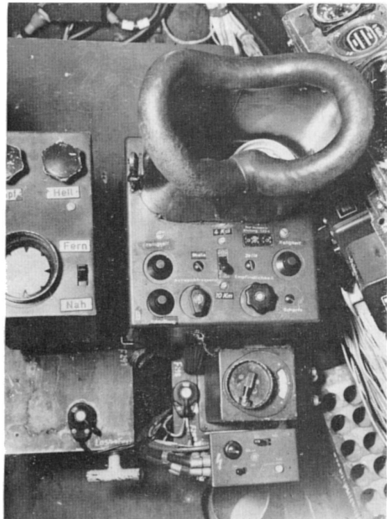
The radio operator's position, showing the indicators for the SN-2 radar (right) and the Naxos homing receiver (left). (Photo: Crown copyright)
