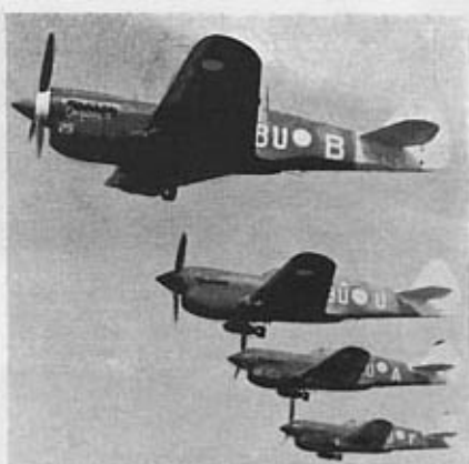
Fine study of Kittyhawk Mk. IV's of No. 80 Sqn., R.A.A.F. with two 500 lb. bombs carried underwing. The nearest aircraft, "Cleopatra III", is a P-40N-20-CU, U.S. serial 43-22834, R.A.A.F. serial A29-629, flown by Group Captain G. C. Atherton. Note white-painted wing leading edges.
