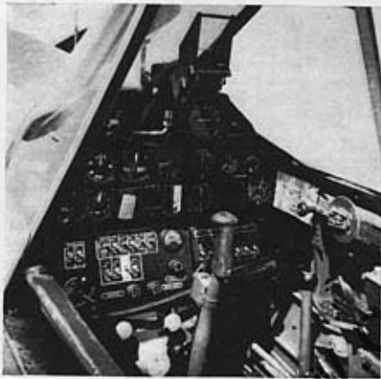
Cockpit and gunsight details of Desert Air Force Kittyhawk Mk. Ia; note operations log under cockpit, showing tally of nine bombing missions and three German aircraft shot down. (Photos via R. Ward)
