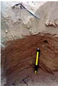
Photo: eg24-21a: Close up of hole showing lower layers of compacted sand which can easily be rubbed away by fingers. The upper 10 cm of sand is loose. All this sand would blow away under appropriate conditions.
